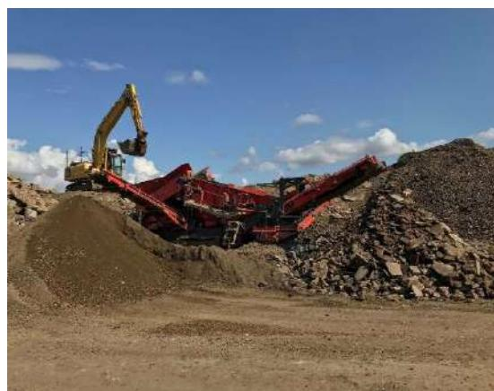
Figure 1 - >50,000 tons of soil waste (filter cake) per annum is processed at the plant in Teesside UK.
