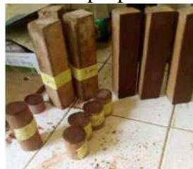
**Illustration:** Geopolymer mortars and concretes.
